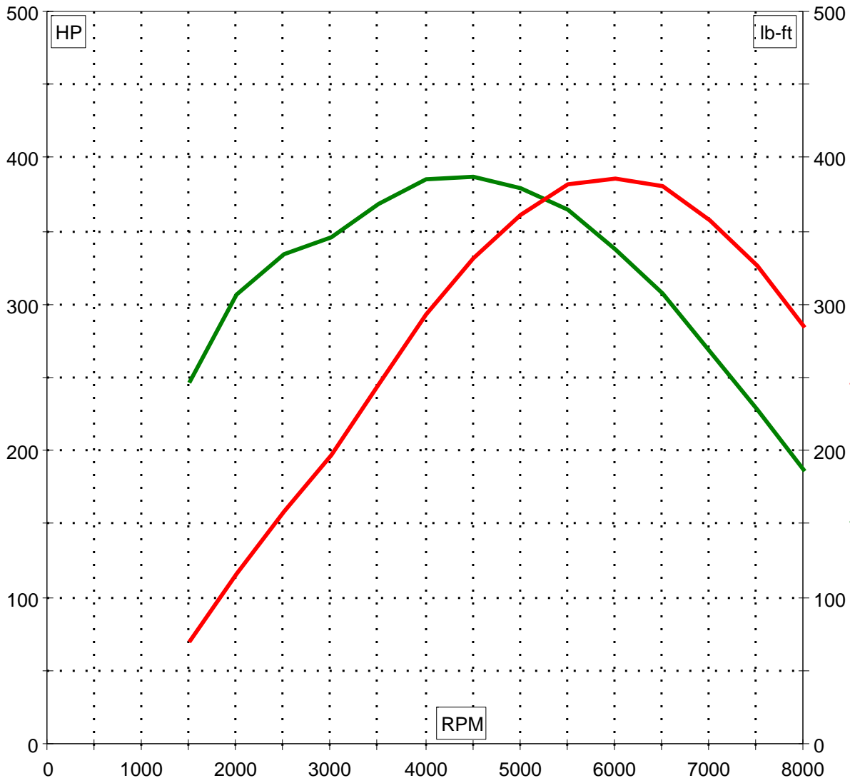
— Power (HP)-BOSS 302 HOWARDS 212241 CAM — Torque (lb-ft)-BOSS 302 HOWARDS 212241 CAM
